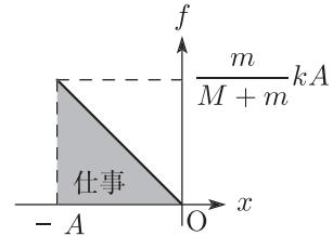
$$\frac{1}{2}mv^2 - 0 = \frac{1}{2} \cdot \frac{m}{M+m}kA^2 \quad \therefore v = A\sqrt{\frac{k}{M+m}}$$
