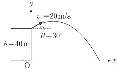
$$(1) \begin{cases} v_x = v_0 \cos \theta = 20 \times \frac{\sqrt{3}}{2} = 10\sqrt{3} \quad \therefore v_x = \underline{10\sqrt{3} [\text{m/s}]} \dots \textcircled{1} \\ v_y = v_0 \sin \theta - gt = 20 \times \frac{1}{2} - 10t = 10 - 10t \quad \therefore v_y = \underline{10 - 10t [\text{m/s}]} \dots \textcircled{2} \end{cases}$$
