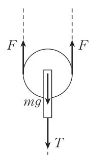
$$F + n + (-Mg) = 0 \cdots ① \quad T + N + (-n) + (-wg) = 0 \cdots ② \quad 2F + (-T) + (-mg) = 0 \cdots ③$$
