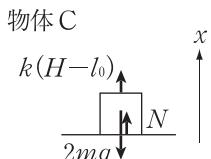
$$k\left(l_0 + \frac{mg}{k} - l_0\right) + N + (-2mg) = 0 \quad \therefore \quad N = \frac{mg}{k}$$
